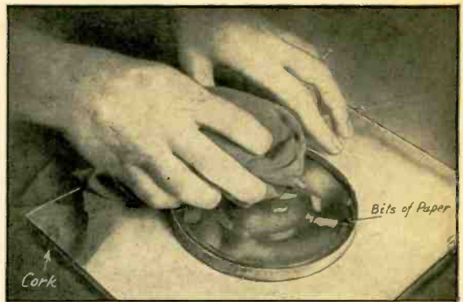
The photo at the left shows a piece of sealing wax attracting small bits of paper after it has been charged by being rubbed with a piece of silk. The photo at the right shows a few bits of paper placed in the lid of a can underneath a piece of dry window glass. When the glass is rubbed briskly with a piece of silk, the pieces of paper will fly to the under surface of the glass and adhere.
