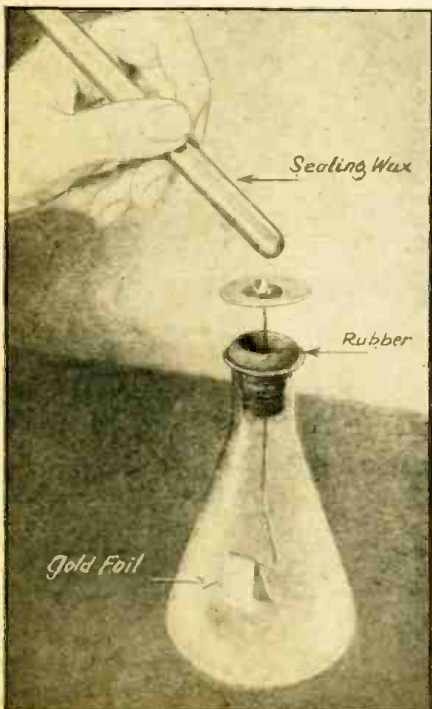
Left—The home-made electroscope in use. When a piece of ordinary sealing wax is rubbed with a silk handkerchief, the leaves of the electroscope will diverge when the end of the wax is brought near. Right—A spark being drawn to the knuckle from a home-made electrophorus.
