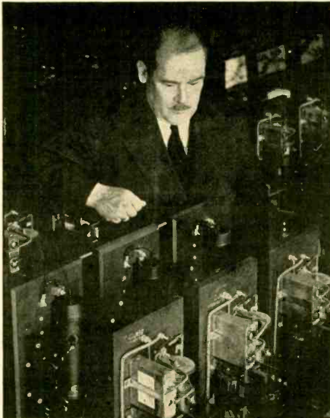
Dr. E. F. W. Alexanderson, G.E. Consulting Engineer, in his laboratory, shown with test set for Thyratron power circuits. Three small metal Thyratron tubes shown on panels immediately in front of him.
