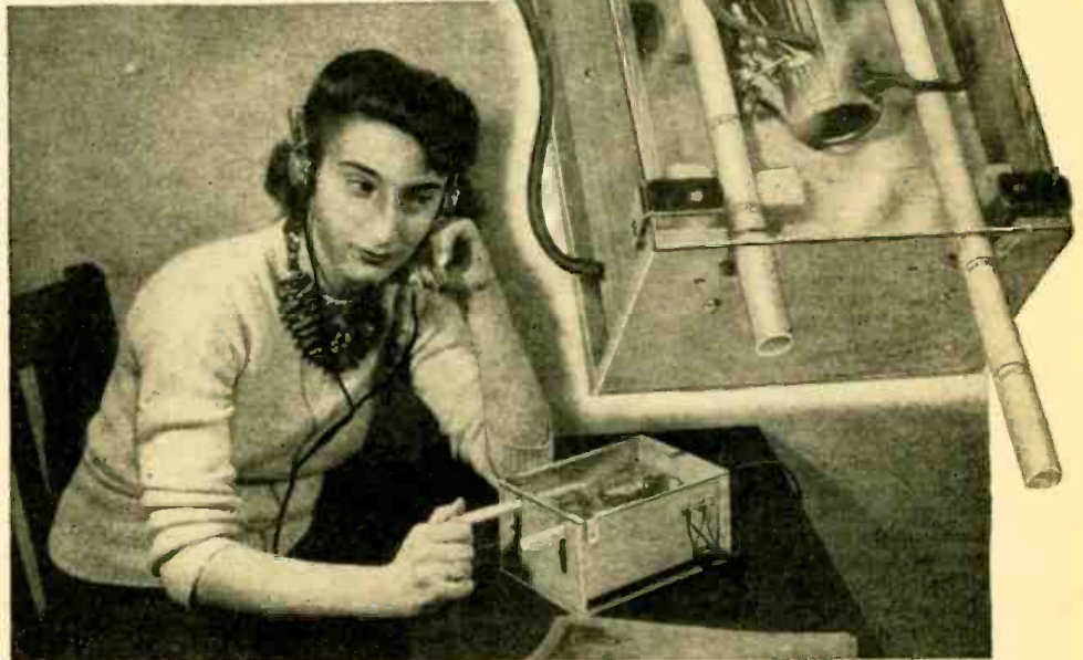
Tuning-up the all-electric model. The control being adjusted is the antenna tuner; the other one is the R.F. plate unit. Ventilation slots at the bottom of the receiver are easily discerned. Note glass cover on receiver.
